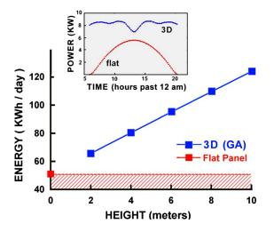
FIG. 1. (Color online) Plot of the energy produced in a day by GAoptimized 3DPV structures compared to that of a flat panel in the same conditions. The inset shows the power generated during the day for the flat panel compared to the 3DPV at height=10 m.
